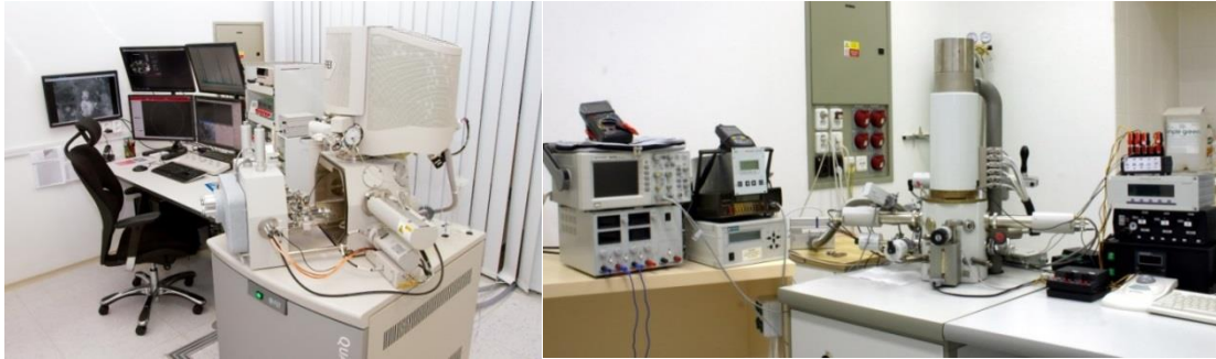
Figure 6.1: New QUANTA 650 FEG environmental scanning electron microscope, equipped with micromanipulators and other unique systems (left) and experimental scanning electron microscope AQUASEM II, rebuilt by the EEM team at ISI CAS in Brno (right).
