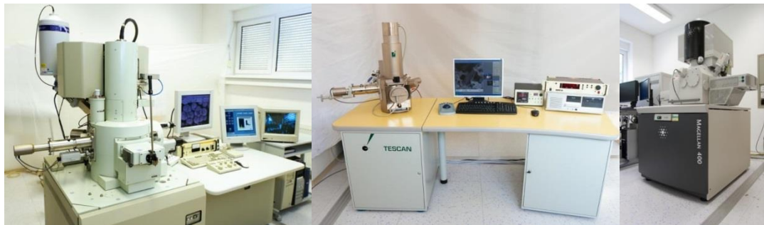
Figure 6.2: The Jeol JSM-6700 high-resolution scanning electron microscope (left), the Vegas robotic scanning electron microscope from Tescan with thermo-emissive cathode (center) and the high-resolution scanning electron microscope MAGELLAN 400 from FEI at ISI CAS in Brno.
