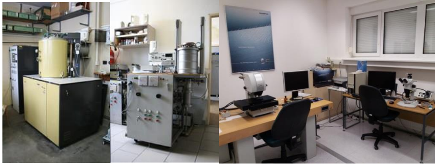
Figure 6.3: Modernized Tesla PZ 810 vertical vacuum furnace (left), small laboratory vacuum furnace (center) and Olympus LEXT OLS3100 optical microscope (right).
